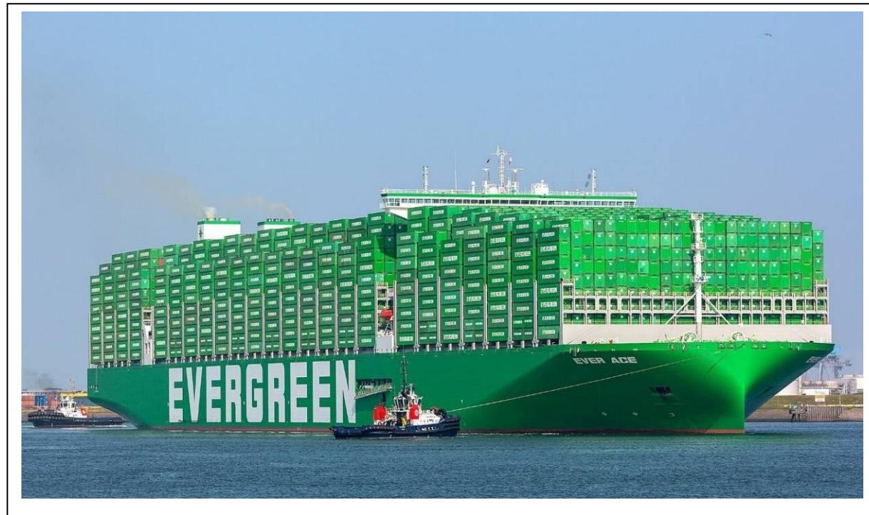
Figure 1. Flattened vertical bow of "EVER ACE" (EVERGREEN, 2021)
